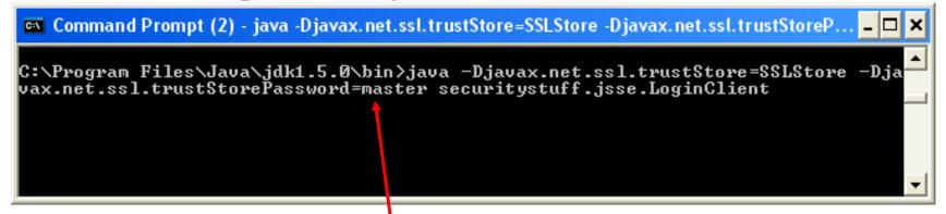
Start the SSL Client application executing with this command where you replace this password with the password you used when you set-up the keystore. Since we are using the same keystore for the server and the client...these will be the same.
